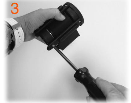
3 Loosen the lower screws slightly on the replacement cassette but do not remove them completely. Do not loosen the top screws.
