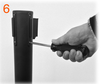
6 Tighten the screws securing the cassette into the post Note: Do not over tighten as this may affect the belt retraction.
