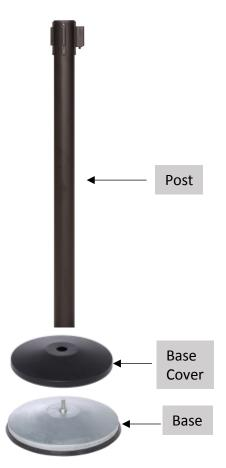
With the base cover in place screw the post onto the base. Make sure the post is screwed down as tightly as possible.
